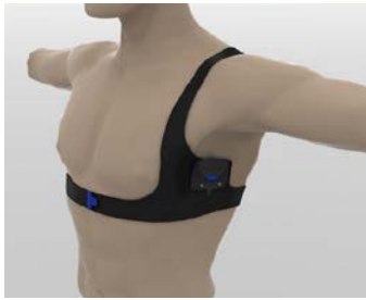
Figure 3. Equivital™ EQ-02 Sensor Electronics Module (SEM) and belt (Equivital Hidalgo, Swavesey Cambridge, UK).
