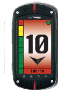
Figure 1. Buddy Display showing a Physiological Strain Index (PSI) of 10 equivalent to extreme thermal-work strain.
