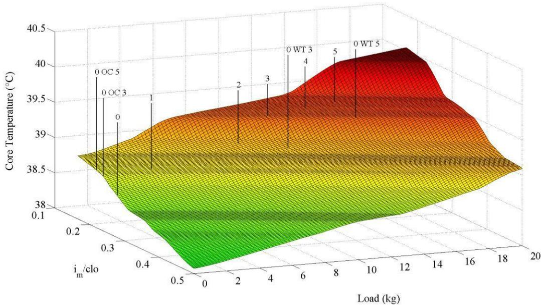
**Figure 5.** Core temperature ( $T_c$ ) transition surfaces viewed from above for body armor protection level (BAPL: 0, 1, 2, 3, 4, 5, 0 WT 3, 0 OC 3, 0 WT 5, 0 OC 5; indicated by “+”) characteristics ( $i_m/clo$  and load) and configurations at 400 and 300 W metabolic rates ( $\dot{M}$ , top and bottom rows) and 50 and 92% relative humidity (RH, left and right columns).
